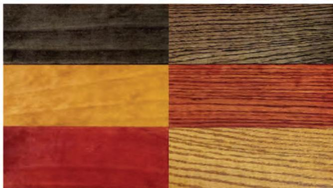
Transparent iron oxides are chemically identical to their opaque counterparts; it is the crystallization process that creates the transparent effect. Extremely durable, light-fast pigments, the UV-curable pigment dispersions shown here showcase the wood grain.
